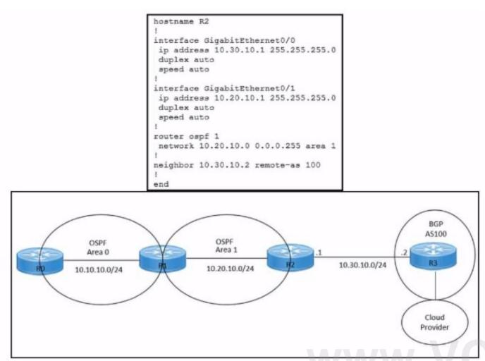
Refer to the exhibits. An engineer must redistribute IBGP routes into OSPF to connect an on-premises network to a cloud provider. Which command must be configured on router R2?
