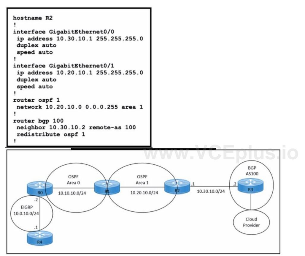
Refer to the exhibits. An engineer must redistribute only the 10.0.10.0/24 network into BGP to connect an on-premises network to a public cloud provider. These routes are currently redistributed: \*10.10.0/24
