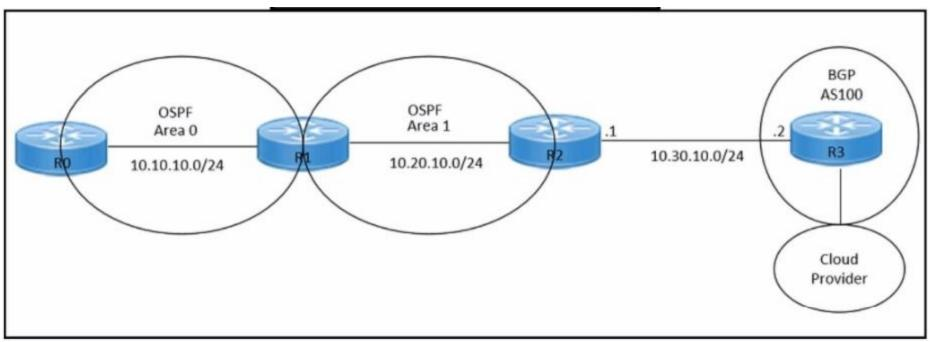
Refer to the exhibits. An engineer must redistribute OSPF internal routes into BGP to connect an on-premises network to a cloud provider. Which two commands should the engineer run on router R2? (Choose two.)
