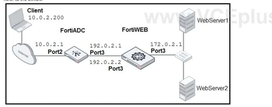
FortiADC is applying SNAT to all inbound traffic going to the servers. When an attack occurs, FortiWeb blocks traffic based on the 192.0.2.1 source IP address, which belongs to FortiADC. The setup is breaking all connectivity and genuine clients are not able to access the servers.
