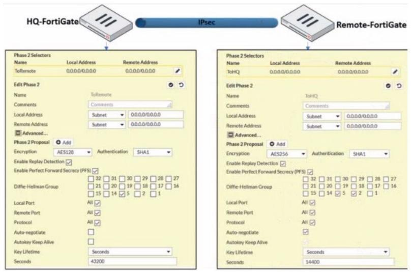
A network administrator is troubleshooting an IPsec tunnel between two FortiGate devices. The administrator has determined that phase 1 status is up. but phase 2 fails to come up. Based on the phase 2 configuration shown in the exhibit, what configuration change will bring phase 2 up?
