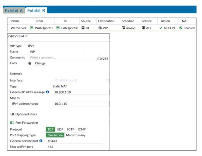
The WAN (port1) interface has the IP address 10.200. 1. 1/24. The LAN (port2) interface has the IP address 10.0. 1.254/24.
