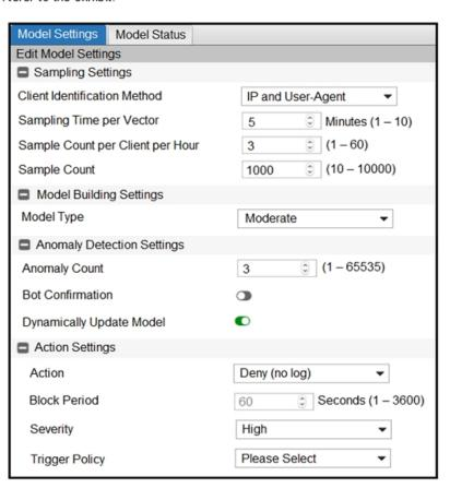
Many legitimate users are being identified as bots. FortiWeb bot detection has been configured with the settings shown in the exhibit. The FortiWeb administrator has already verified that the current model is accurate.
