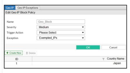
FortiWeb is configured to block traffic from Japan to your web application server. However, in the logs, the administrator is seeing traffic allowed from one particular IP address which is geo-located in Japan.
