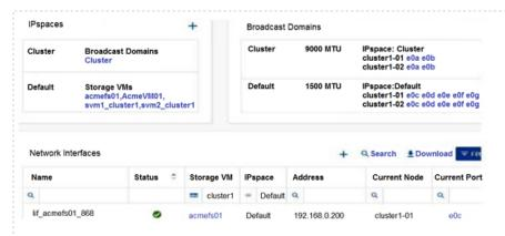
You have an ONTAP 9.8 cluster. After network maintenance, the LIF that is shown in the exhibit is not always on a correct port and is unreachable by users until the LIFs are moved to port e0c or e0d on either storage node.
