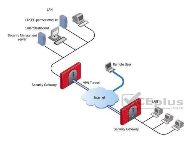
Assume an environment with gateways on different sites. Each Security Gateway connects to the Internet on one side, and to a LAN on the other.
