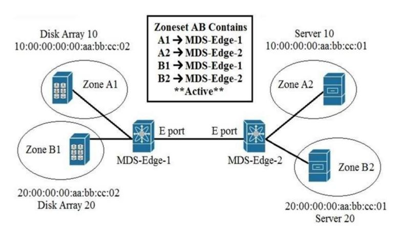
An engineer is implementing zoning on two Cisco MDS switches. After the implementation is finished, E Ports that connect the two Cisco MDS switches become isolated.
