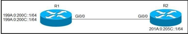
ipv6 access-list Deny\_Telnet sequence 10 deny tcp host 198A:0:200C::1/64 host 201A:0:205C::1/64 eq telnet ! int Gi0/0 ipv6 traffic-filter Deny\_Telnet in !
