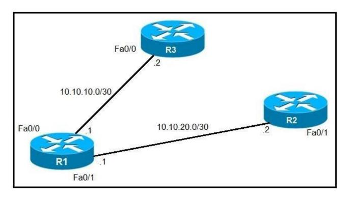
Refer to the exhibit. An IP SLA was configured on router R1 that allows the default route to be modified in the event that Fa0/0 loses reachability with the router R3 Fa0/0 interface. The route has changed to flow through router R2.
