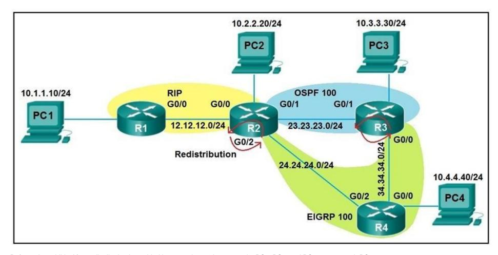
Refer to the exhibit. After redistribution is enabled between the routing protocols; PC2, PC3, and PC4 cannot reach PC1.
