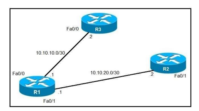
Refer to the exhibit. An IP SLA was configured on router R1 that allows the default route to be modified in the event that Fa0/0 loses reachability with the router R3 Fa0/0 interface. The route has changed to flow through router R2. Which debug command is used to troubleshoot this issue?
