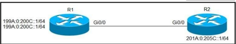
ipv6 access-list Deny\_Telnet sequence 10 deny tcp host 198A:0:200C::1/64 host 201A:0:205C::1/64 eq telnet ! int Gi0/0 ipv6 traffic-filter Deny\_Telnet in !
