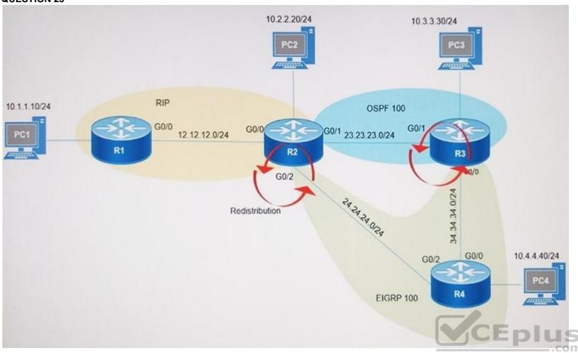
Refer to the exhibit. After redistribution is enabled between the routing protocols; PC2, PC3, and PC4 cannot reach PC1. Which action can the engineer take to solve the issue so that all the PCs are reachable?
