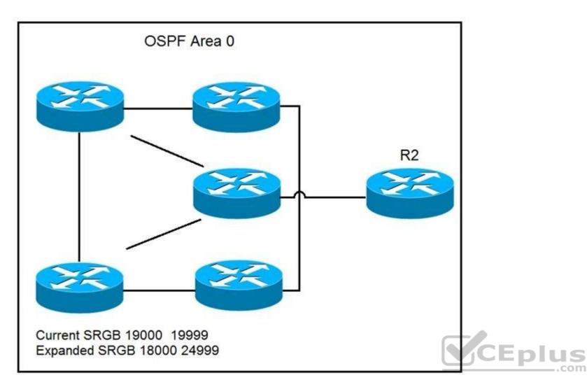
Refer to the exhibit. A network operator wants to expand the segment routing global block in upcoming maintenance. The operator must ensure that the changes to the segment routing global block have no adverse impacts on the prefix-sid associated with the loopback0 interface used within the OSPF domain. Which command can the operator use to enforce R2 to have a strict prefix-sid assignment to loopback0? A.
