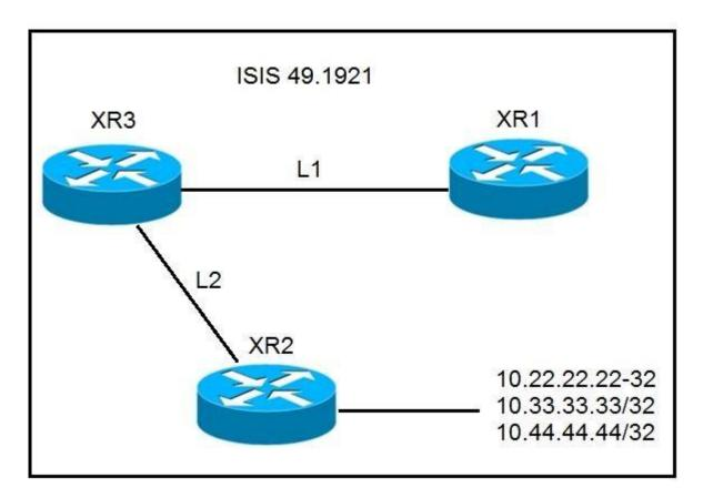
Refer to the exhibit. A network operator must stop 10.33.33.33/32 from being redistributed into Level 1 router XR1. Which configuration meets this need? A.
