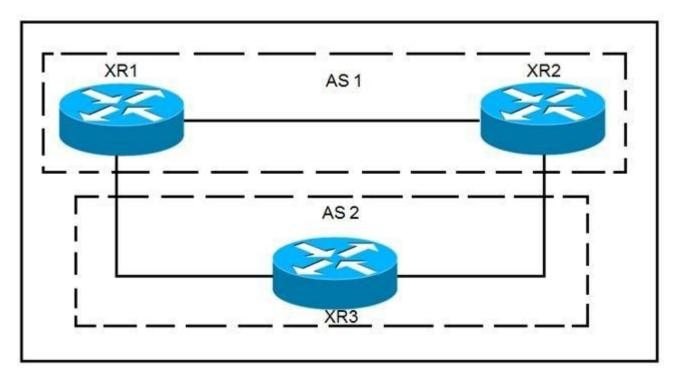
Refer to the exhibit. XR1 and XR2 are sending the prefix 10.11.11.0/24 to XR3. A configured policy on XR1 is incorrectly prepending AS path 11 11 12 12 onto this prefix. A network operator wants to add a policy onto XR3 that will not allow the falsely prepending prefix from being installed. Which policy configuration applied to the XR3 neighbor configuration for XR1 can accomplish this requirement without impact to other or future received routes? A.
