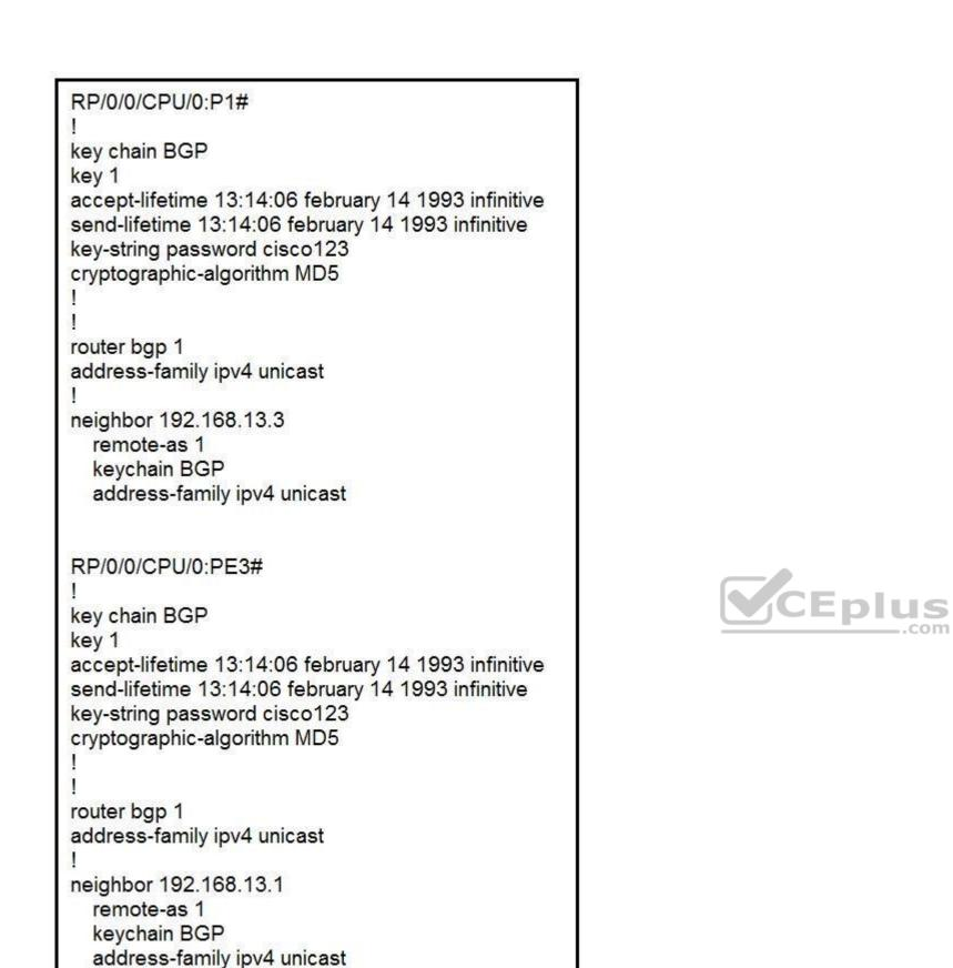
Refer to the exhibit. P1 and PE3 Cisco IOS XR routers are directly connected and have this configuration applied. The BGP session is not coming up. Assume that there is no IP reachability problem and both routers can open tcp port 179 to each other. Which two actions fix the issue? (Choose two.)
