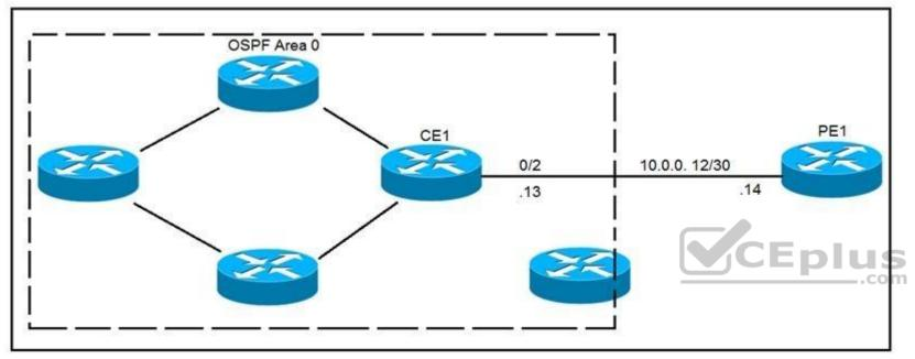
Refer to the exhibit. CE1 is the gateway router into the provider network via PE1. A network operator must inject a default route into OSPF area 0. All devices inside area 0 must be able to reach PE1. Which configuration achieves this
