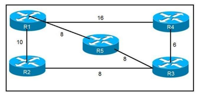
Refer to the exhibit. Which router does R1 install as an alternate next hop when trying to reach R3 if LFA is enabled?
