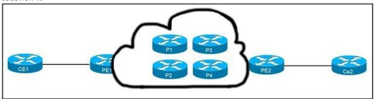
Refer to the exhibit. CE1 and CE2 cannot communicate through the service provider BGP peering is established between PE1 and PE2. IS-IS is the only routing protocol running in the service provider core. What step can be done to troubleshoot the issue?
