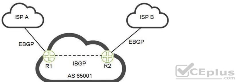
You are configuring BGP policies for a site with a dual-homed connection as shown in the exhibit. You must ensure that inbound traffic from Internet hosts flow through the ISP A connection.
