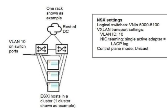
The exhibit indicates the customer NSX design and your plan for the connected ToR switches, which are ArubaOS-CX switches.
