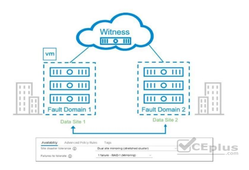
A storage administrator is designing a vSAN stretched cluster with production workload running on a preferred site. A VM has been deployed on the preferred site. How does the VM read I/O?
