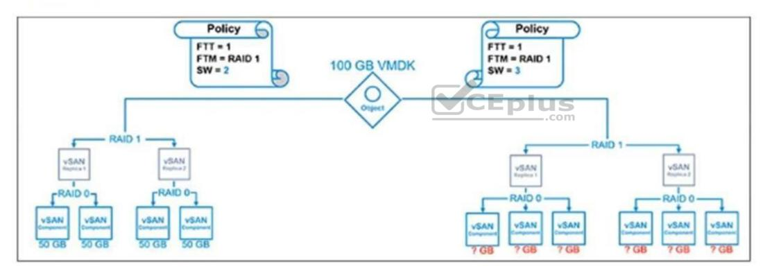
In a 2-node vSAN environment, a storage administrator has setup a vSAN storage policy. When the stripe width is changed to three, what is the approximate size of each replica marked in red?
