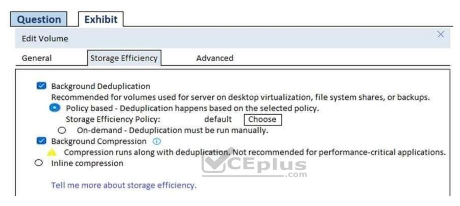
You have a performance critical database application that is running on a FAS9000 controller that uses FC. As shown in the exhibit, volume efficiency is enabled.
