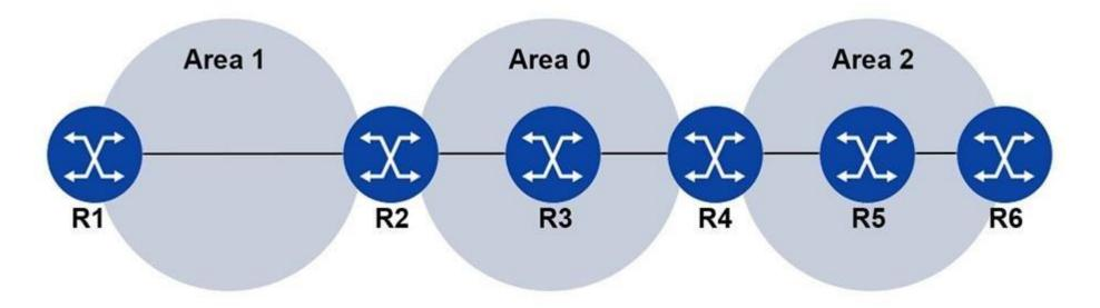
A. Router R3 swaps both the RSVP-TE LSP label and LDP transport label received with new labels.
