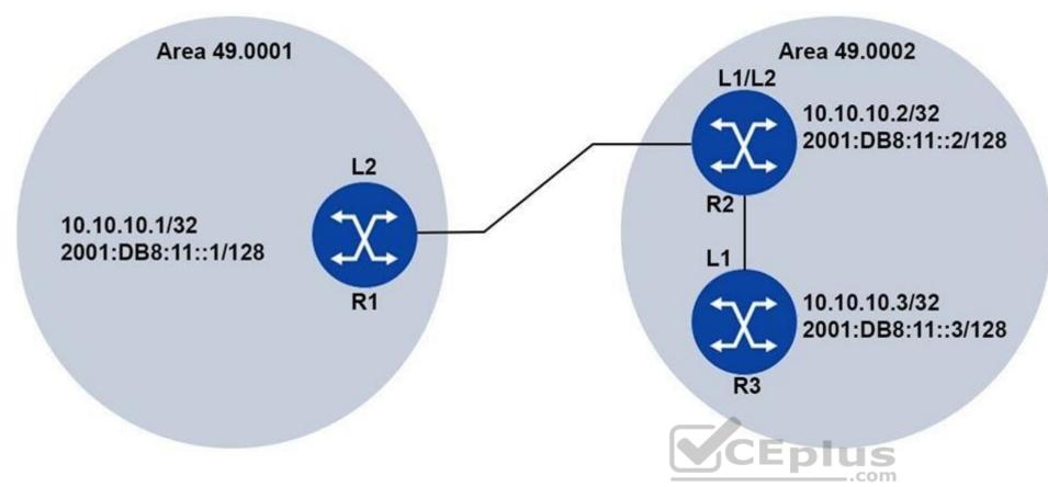
The routers have established IS-IS adjacencies on which IPv4 system addresses are exchanged. An operator successfully configures multi-topology IS-IS routing so that the IPv6 system addresses are also exchanged between routers. After IPv6 has been configured, which of the following is TRUE?
