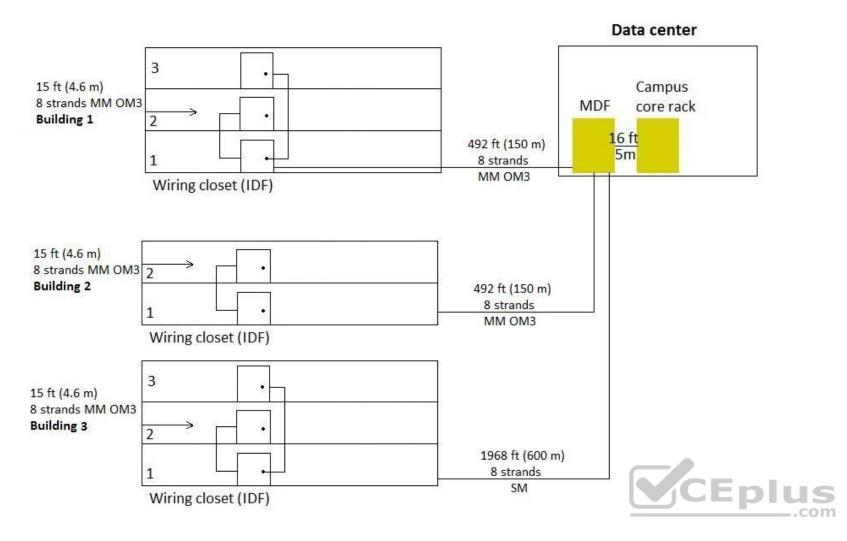
An architect needs to design the topology for a new wired network at a campus with three buildings. The exhibit above shows the cabling layout.
