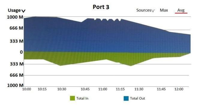
A customer needs a wired network upgrade and has complained about performance issues. The architect has collected information about traffic flow on several switch ports in different locations across the network, and the results are shown in the exhibit. Each of these ports is a 1Gbps port. What can the architect conclude?
