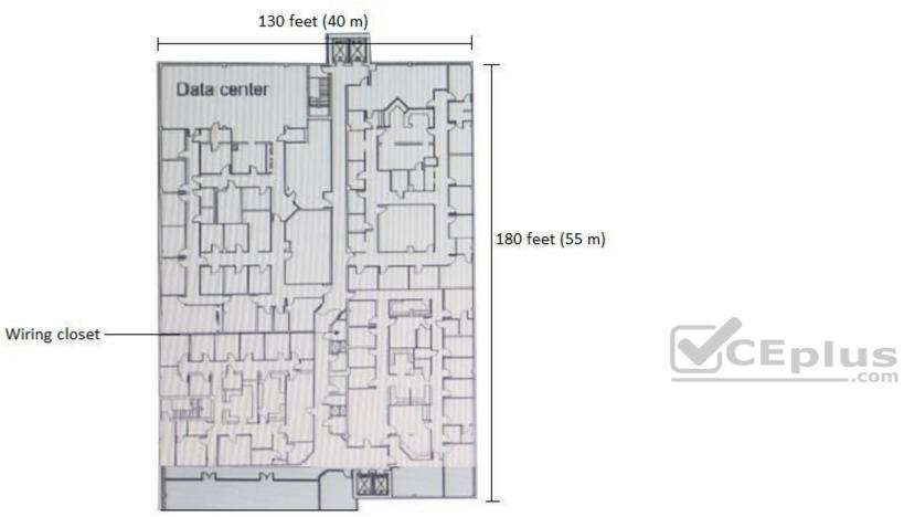
The customer requires a solution for the writing closet shown in the exhibit. The closet serves the entire floor, which is wired for CAT5e cable. The closet has four CAT5e cables to the data center 110 feet (34 m) away. The switch or switches in this closet will need to support 100 wired endpoints and 16 AP-345s. The switch or switches must connect to the network core, Aruba 5406R switches, in the data center on uplinks that provide at least 20 Gbps bandwidth total.
