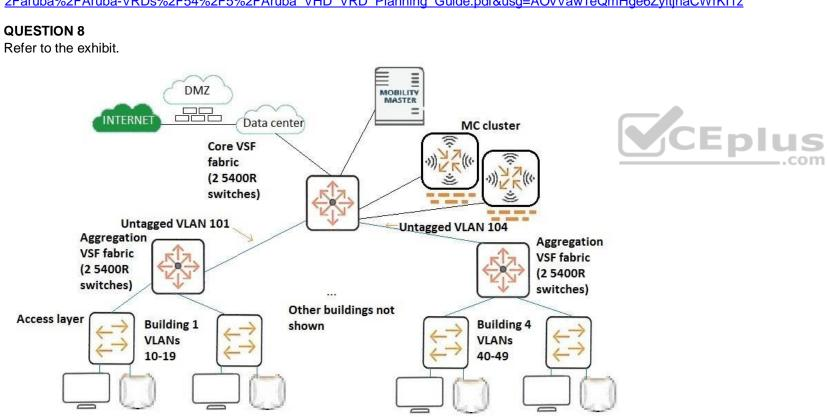
A customer has a wired infrastructure shown in the exhibit. The customer is in the process of expanding their wireless services. They will now add a new wireless solution, with mobility controllers (MCs) connected as shown. The new wireless solution will support a total of 450 APs and about 26,000 wireless devices. It must provide seamless roaming across the entire campus. After the new deployment, both wired and wireless devices experience IP connectivity issues.
