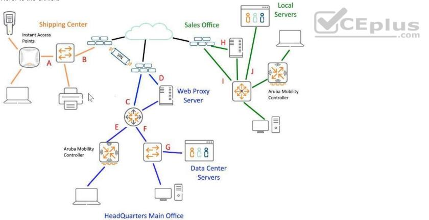
Given the network diagram, would this be a proper location for a network tap? (Port G at the Head Quarters Site would expose all East/West traffic bound for the data center.)
