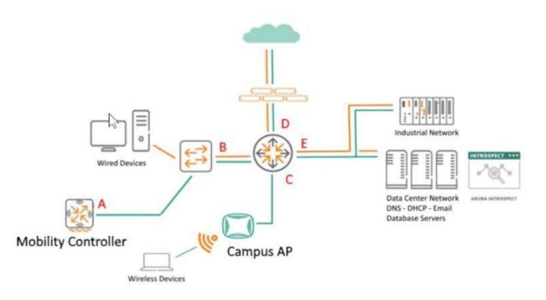
You are monitoring network traffic and considering DNS flow patterns. Where is a good location to place the Network Tap or Taps? (Location D will capture all DNS requests.)
