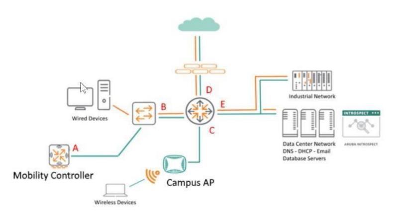
You are monitoring network traffic and considering DNS flow patterns. Where is a good location to place the Network Tap or Taps? (Location A.)
