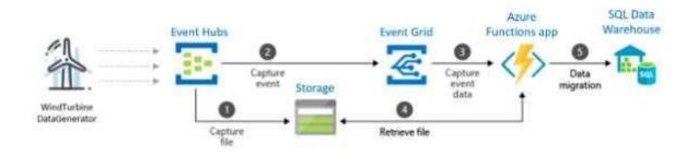
First, you create an event hub with the Capture feature enabled and set an Azure blob storage as the destination. Data generated by WindTurbineGenerator is streamed into the event hub and is automatically captured into Azure Storage as Avro files.
