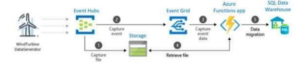
First, you create an event hub with the Capture feature enabled and set an Azure blob storage as the destination. Data generated by WindTurbineGenerator is streamed into the event hub and is automatically captured into Azure Storage as Avro files.
