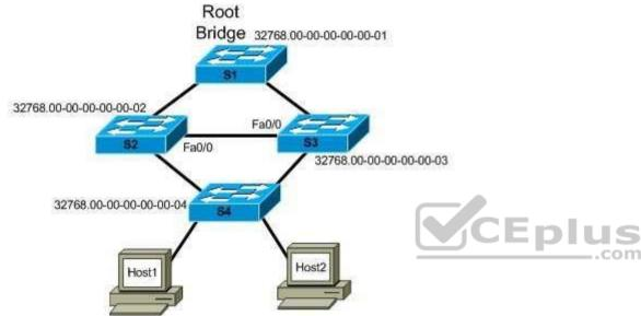
You administer the network shown in the exhibit above. You enable root guard by issuing the spanning-tree guard root command in interface configuration mode for the Fa0/0 interfaces of S2 and S3.
