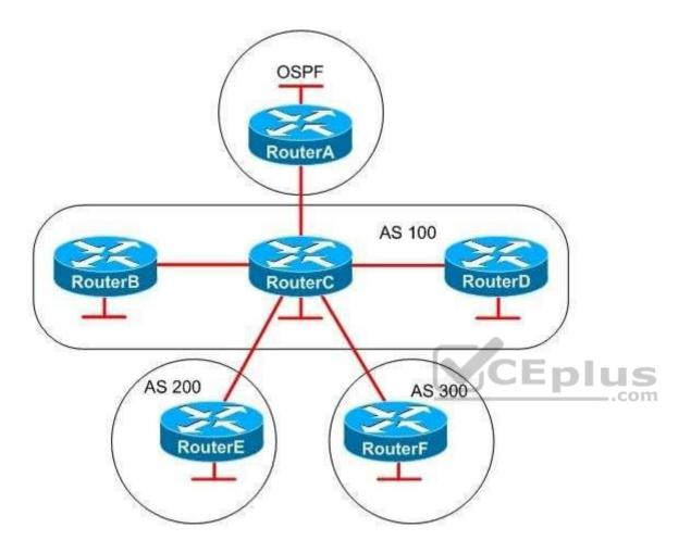
You administer the networks shown above. RouterA is connected to network A, RouterB is connected to network B, and so on. RouterB and RouterD are iBGP peers of RouterC; RouterE and RouterF are eBGP peers of RouterC. RouterA and RouterC are OSPF neighbors.
