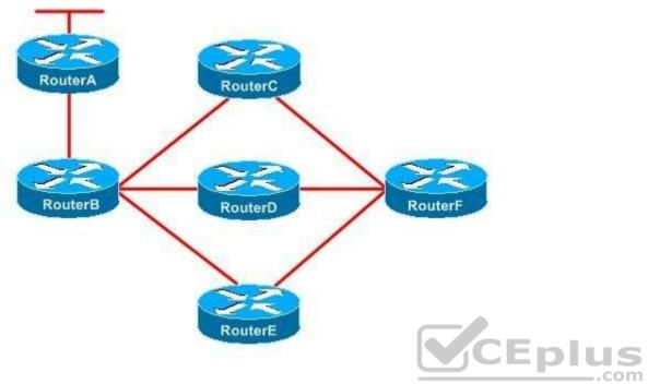
You administer the EIGRP network shown above. RouterB is configured to send only a summary route to RouterE. RouterC is configured as a stub router. The link between RouterA and RouterB fails.
