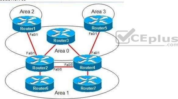
You administer the OSPF network shown in the diagram. Area 1 is configured as a standard area. Area 2 and Area 3 are configured as stub areas. Router3 fails. Several routes are lost throughout the network.
