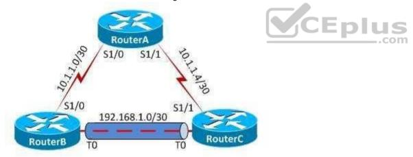
All routers are configured to the system MTU defaults. You issue the ping 192.168.1.2 size 1500 dfbit command from RouterB, but the ping fails. Which of the following is most likely the cause of the failure? (Select the best answer.)
