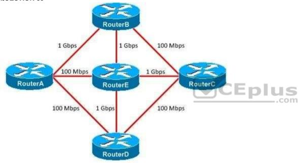
You administer the OSPF network shown in the diagram above. The reference bandwidth has been changed to 1000 on every router in the network. What is the cost of the route from RouterA to RouterC? (Select the best answer.)
