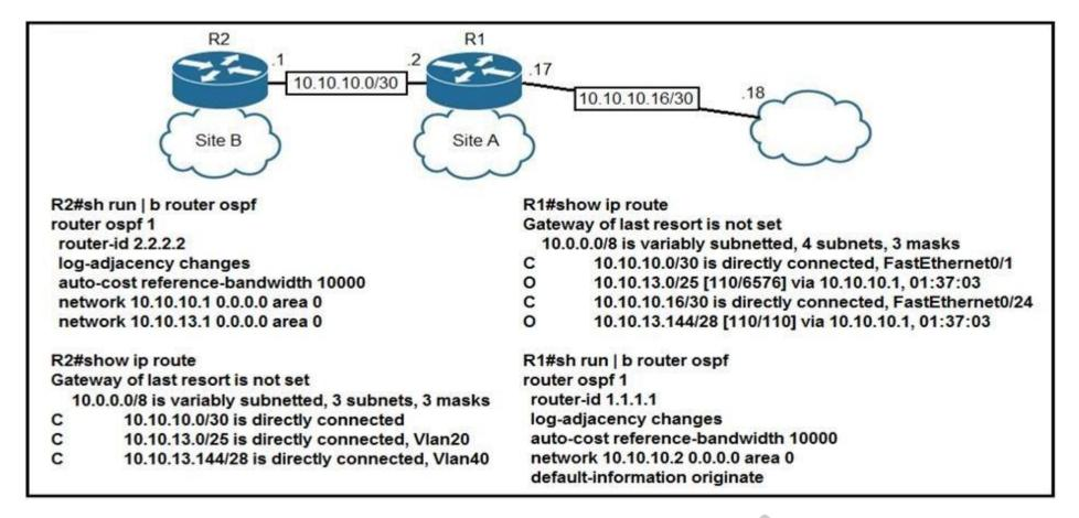
Refer to the exhibit. The default-information originate command is configured under the R1 OSPF configuration. After testing, workstations on VLAN 20 at Site B cannot reach a DNS server on the Internet.
