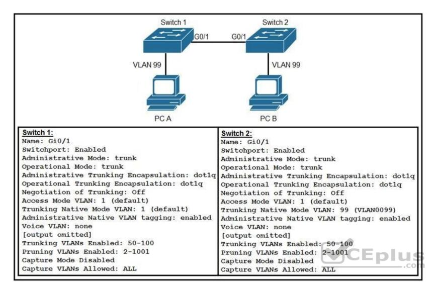
Refer to the exhibit. After the switch configuration, the ping test fails between PC A and PC B. Based on the output for switch 1, which error must be corrected?
