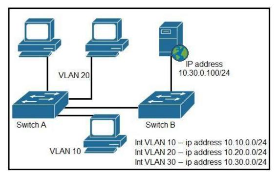
Refer to the exhibit. A network engineer must block access for all computers on VLAN 20 to the web server via HTTP. All other computer must be able to access the web server. Which configuration when applied to Switch A accomplishes the task? A.
