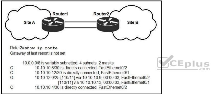
Refer to the exhibit. If OSPF is running on this network, how does Router2 handle traffic from Site B to 10.10.13.128/25 at Site A?
