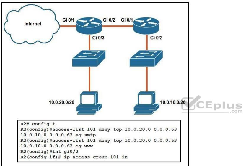
Refer to the exhibit. An extended ACL has been configured and applied to router R2. The configuration failed to work as intended.
