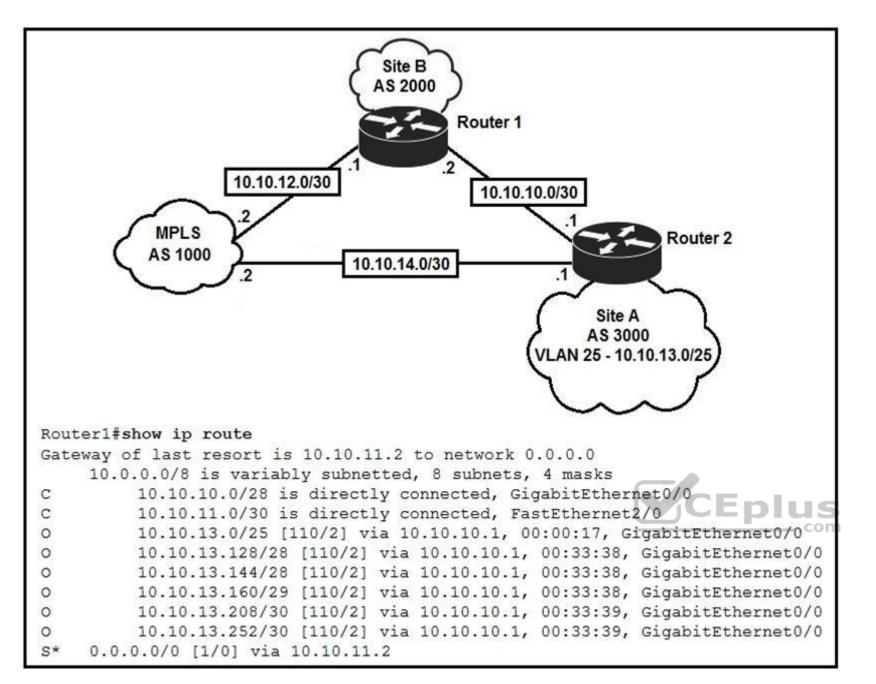
Refer to the exhibit. An engineer is bringing up a new circuit to the MPLS provider on the Gi0/1 interface of Router 1. The new circuit uses eBGP and learns the route to VLAN25 from the BGP path.
