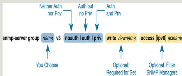
**Figure D-13** *SNMPv3 Groups—Configuration Command Parameters*
