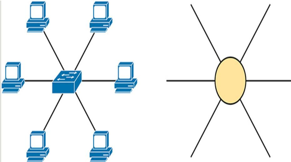
**Figure 13-2** *The Star Topology Design Concept in Networking*
