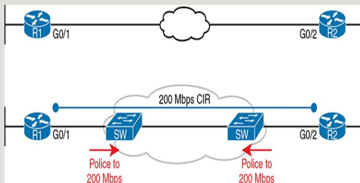
**Figure 11-19** *Ethernet WAN: Link Speed Versus CIR*
