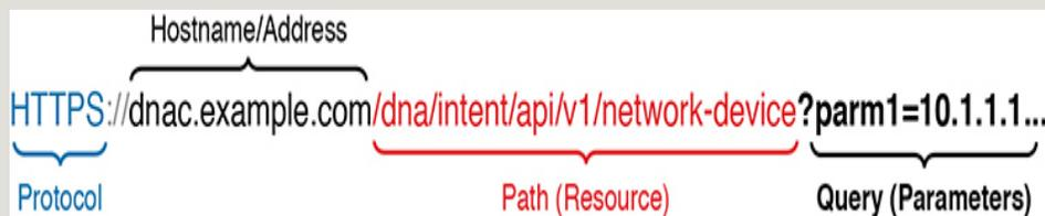
**Figure 18-8** *Example Components of a URI Used in a REST API Call*
