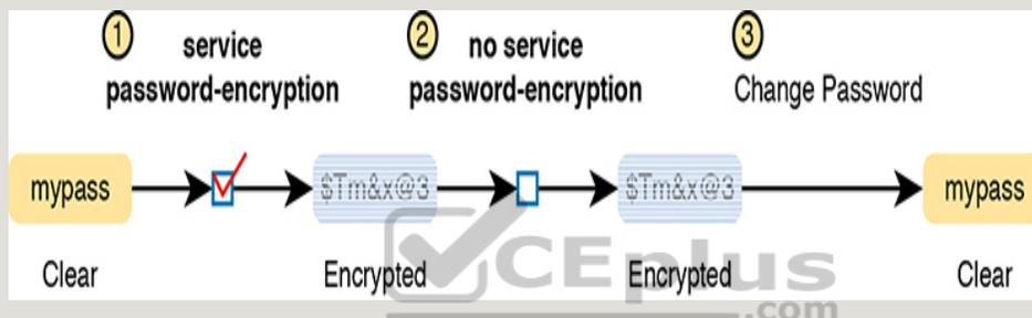
**Figure 5-2** *Encryption Is Immediate; Decryption Awaits Next Password Change*
