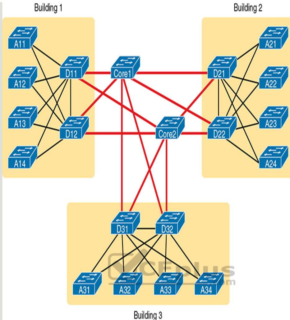
**Figure 13-5** *Three-Tier Building Design (Core Design), Three Buildings*
