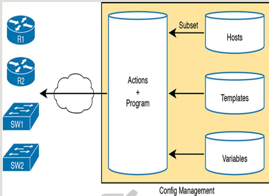
**Figure 19-7** *Important Files Used by Configuration Management Tools*
