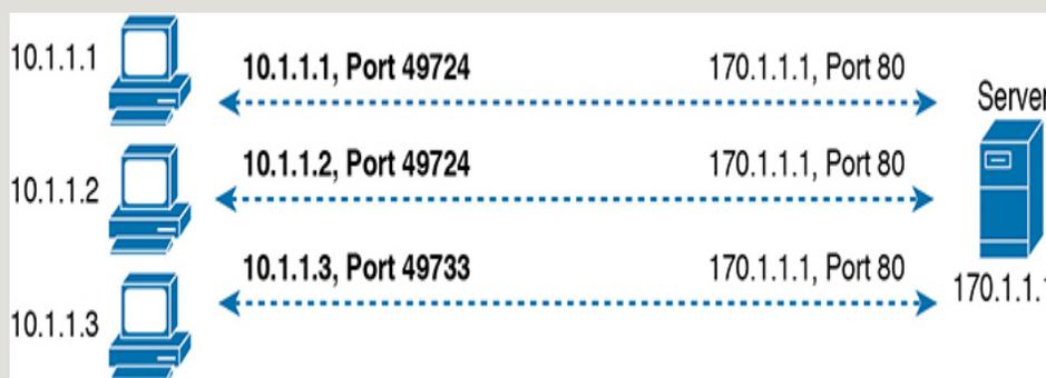
**Figure 10-6** *Three TCP Connections from Three PCs*
