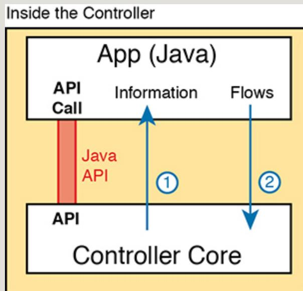
**Figure 16-6** *Java API: Java Applications Communicates with Controller*
