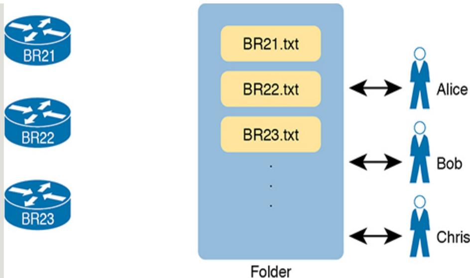
**Figure 19-2** *Copying Device Configurations to a Central Location*
