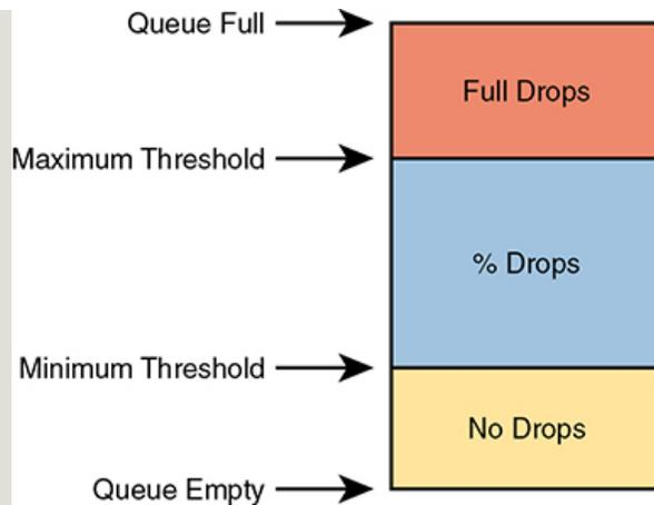
**Figure 11-23** *Mechanisms of Congestion Avoidance*
