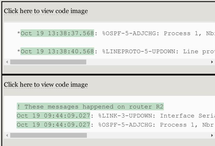
In reality, the messages in both parts of Example 9-6 happened within 0.5 seconds of each other because I issued a **shutdown** command on one of the routers. However, the two routers' time-of-day clocks were not synchronized, which makes the messages on the two routers look unrelated. With synchronized clocks, the two routers would have listed practically identical timestamps of almost the exact same time when these messages occurred, making it much easier to read and correlate messages.
