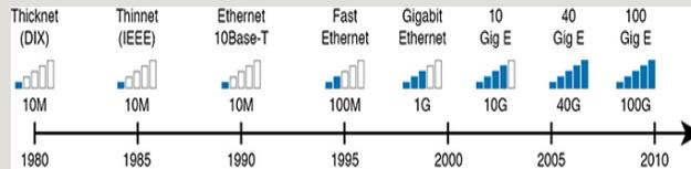
**Figure D-17** Ethernet Standards Timeline
