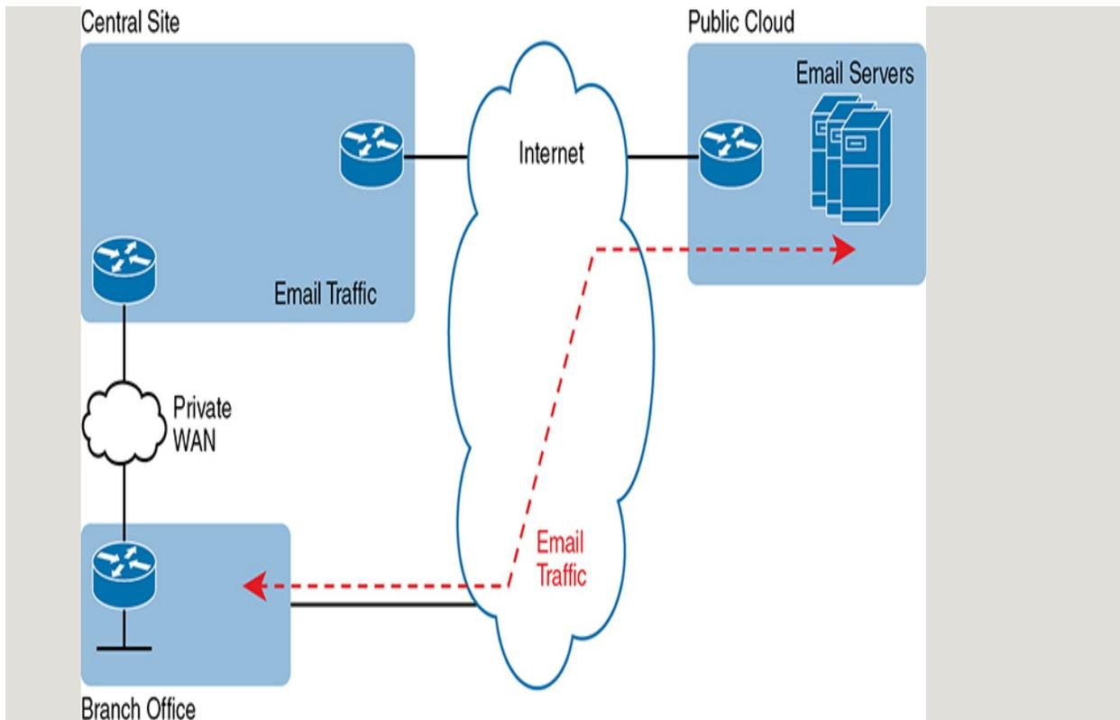
**Figure 15-18** *Connecting Branches Directly to the Internet for Public Cloud Traffic*
