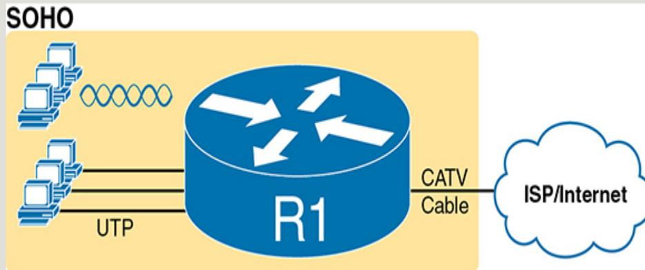
**Figure 13-7** *A Typical Home Wired and Wireless LAN*
