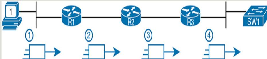
**Figure 16-1** *Data Plane Processing on Routers: Basics*
