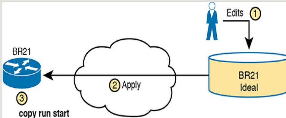
**Figure 19-4** *Pushing Centralized Configuration to a Remote Device*
