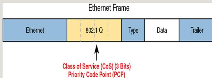
**Figure 11-7** *Class of Service Field in 802.1Q/p Header*
