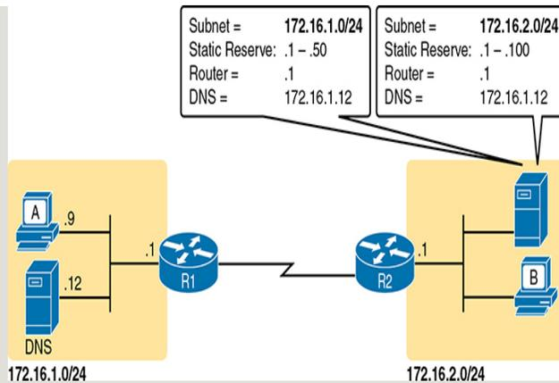
**Figure 7-4** Preconfiguration on a DHCP Server
