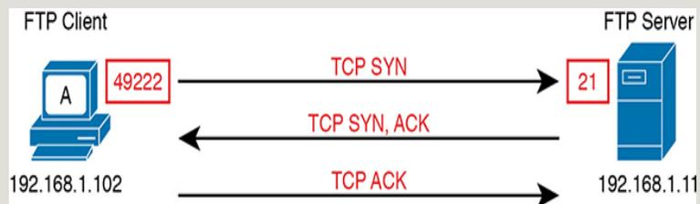
**Figure 12-17** *FTP Client Creates an FTP Control Connection*
