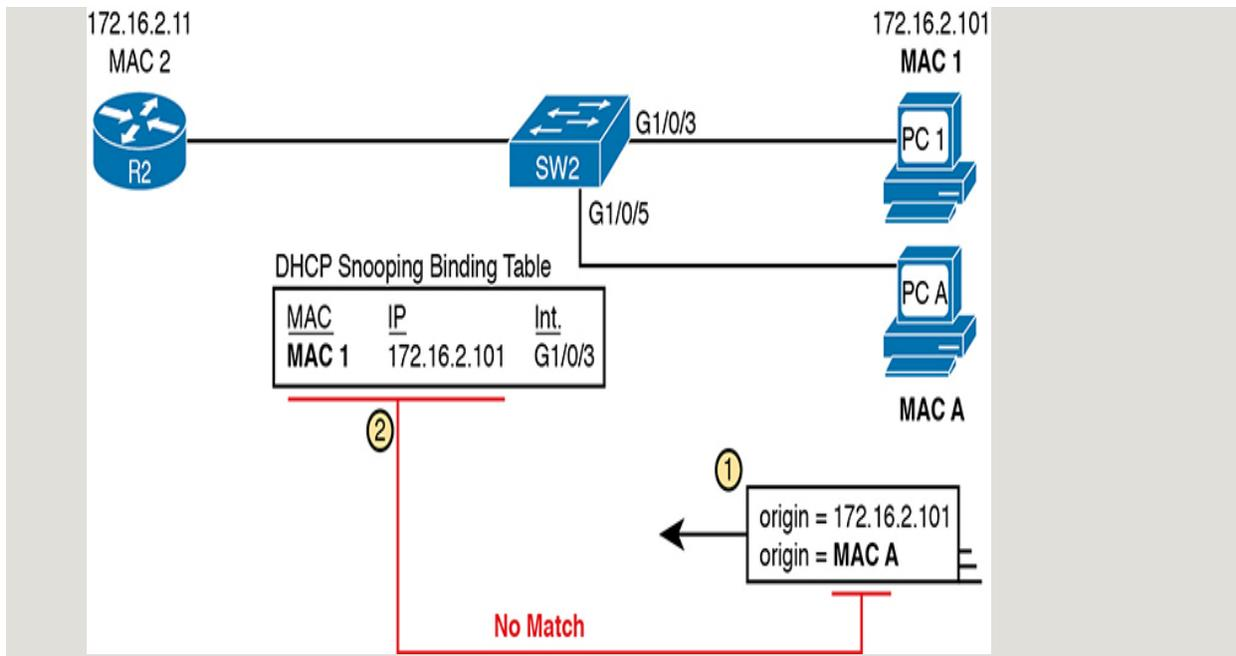
**Figure 8-13** *DAI Filtering ARP Based on DHCP Snooping Binding Table*
