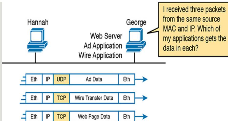
**Figure 1-2** *Hannah Sending Packets to George, with Three Applications*
