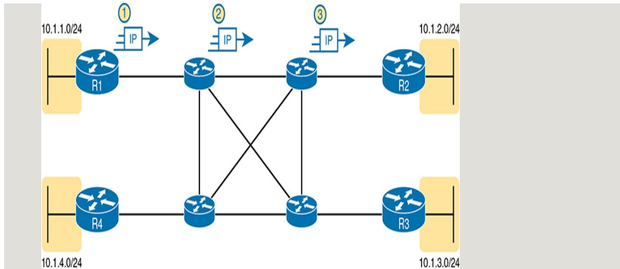
**Figure 14-10** *Basic IP Routing of IP Packets*
