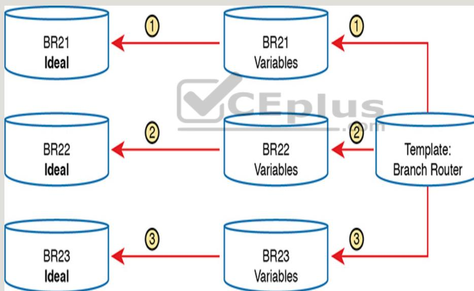
**Figure 19-6** *Concept: Configuration Templates and Variables*
