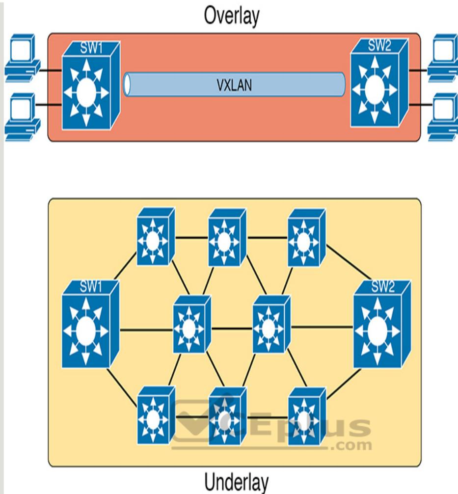
**Figure 17-2** *Fabric, Underlay, and Overlay Concepts*
