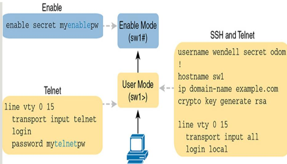
**Figure 5-1** Sample Login Security Configuration
