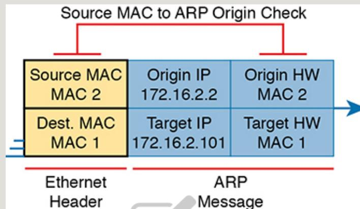
**Figure 8-14** *DAI Filtering Checks for Source MAC Addresses*
