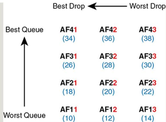
**Figure 11-11** *Differentiated Services Assured Forwarding Values and Meaning*
