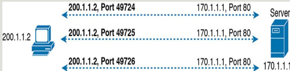
**Figure 10-7** *Three TCP Connections from One PC*
