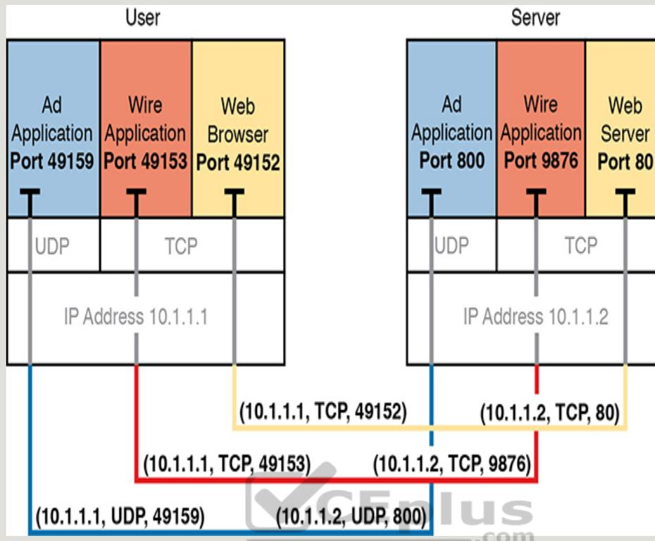
**Figure 1-4** *Connections Between Sockets*
