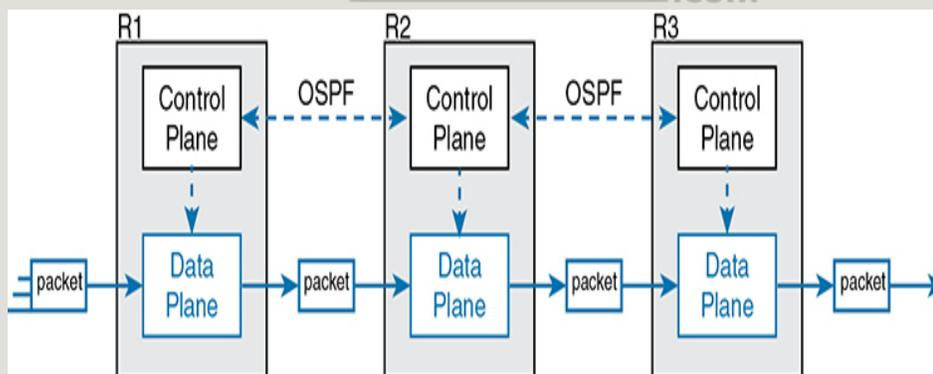
**Figure 16-2** *Control and Data Planes of Routers—Conceptual*
