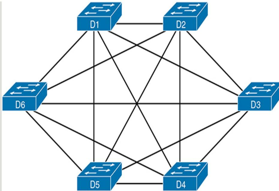
**Figure 13-3** *Using a Full Mesh at the Distribution Layer, 6 Switches, 15 Links*
