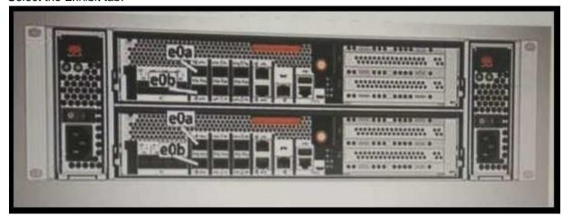
Your customer has an AFF A300 installed. They ask you to configure the e0a and e0b ports to use the FC protocol.
