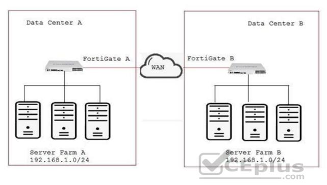
Your company has two data centers (DC) connected using a Layer 3 network. Servers in farm A need to connect to servers in farm B as though they all were in the same Layer 2 segment. What would be configured on the FortiGates on each DC to allow such connectivity?
