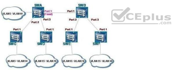
As shown in the figure, port 1 of switch A is configured with the Fixed mode, and other ports are configured with the Normal mode. The trunk interfaces allow all VLANs. Which VLANs are registered on port 1 of switch C? (Select 3 Answers)
