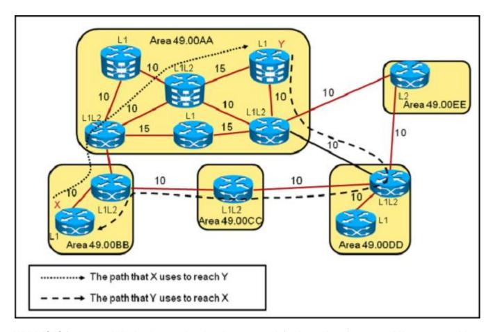
Which IS-IS feature could be implemented so that the return path for the packets from router Y in area 49.00AA to router X in area 49.00BB will use the more optimal path?
