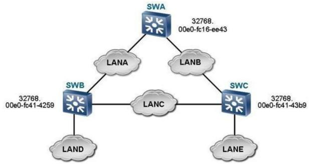
As shown in the figure, which switch is the root switch according to the configuration?
