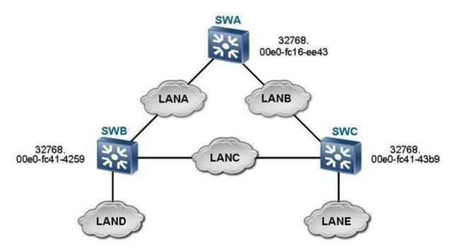
On the STP network as shown in the figure, which device may be the blocked port belong to?
