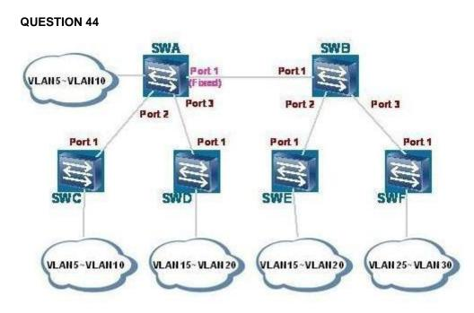
As shown in the figure, port 1 of switch A is configured with the Fixed mode, and other ports are configured with the Normal mode. The trunk interfaces allow all VLANs. Which VLANs are registered on port 1 of switch C? (Select 3 Answers)
