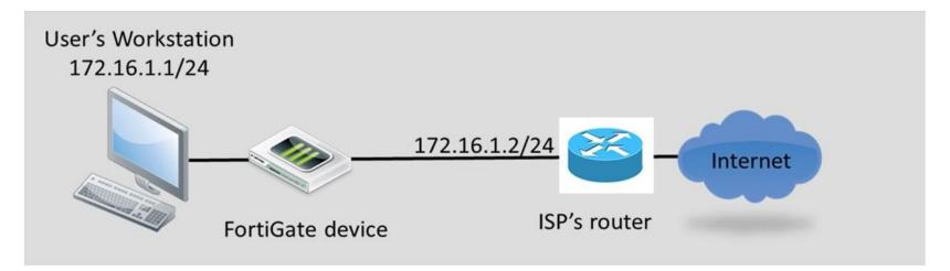
The workstation, 172.16.1.1/24, connects to port2 of the FortiGate device, and the ISP router, 172.16.1.2, connects to port1. Without changing IP addressing, which configuration changes are required to properly forward users traffic to the Internet? (Choose two)
