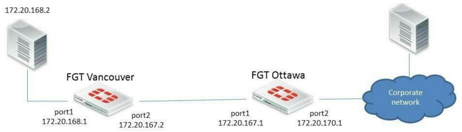
In this scenario. The FortiGate unit in Ottawa has the following routing table:
