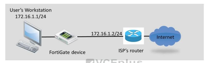
The workstation, 172.16.1.1/24, connects to port2 of the FortiGate device, and the ISP router, 172.16.1.2, connects to port1. Without changing IP addressing, which configuration changes are required to properly forward users traffic to the Internet? (Choose two)
