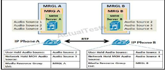
All displayed devices are registered to the same Cisco Unified Communications Manager server and the phones are engaged in an active call. Assuming the provided configurations exist at the phone line level and multicast MOH is disabled clusterwide, what will happen when the user of IP Phone B presses the Hold softkey?
