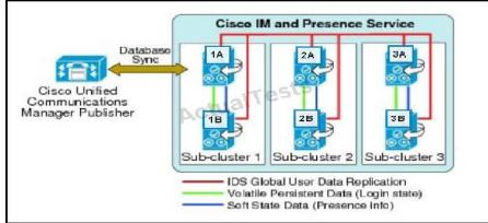
In this high-availability Cisco IM and Presence deployment with three subclusters, the first user is assigned to server 1A; the second user is assigned to server 2A; and the third user is assigned to
