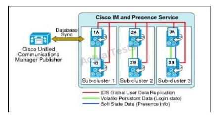
In this high-availability Cisco IM and Presence deployment with three subclusters, the first user is assigned to server 1A; the second user is assigned to server 2A; and the third user is assigned to server 3A. Assume that the Cisco IM and Presence is set to Active/Standby mode, to which server should the fourth user be assigned?
