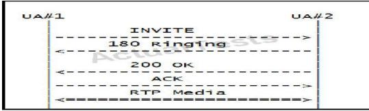
If this SIP call is initiated using delayed offer, which SIP message will UA#1 use to communicate its media capability to UA#2?
