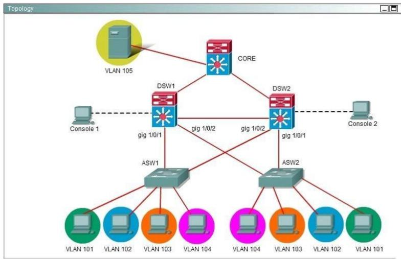
All interfaces are active. DSW2 has not become the active device for the VLAN 103 HSRP group. As related to the VLAN 103 HSRP group, what can be done to make the group function properly?
