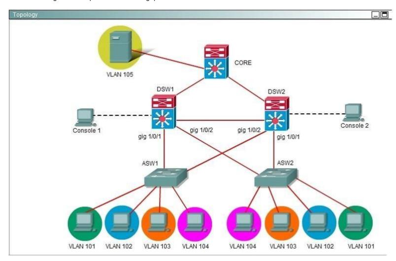
During routine maintenance, it became necessary to shut down the GigabitEthernet1/0/1 interface on DSW1 and DSW2. All other interfaces were up.
