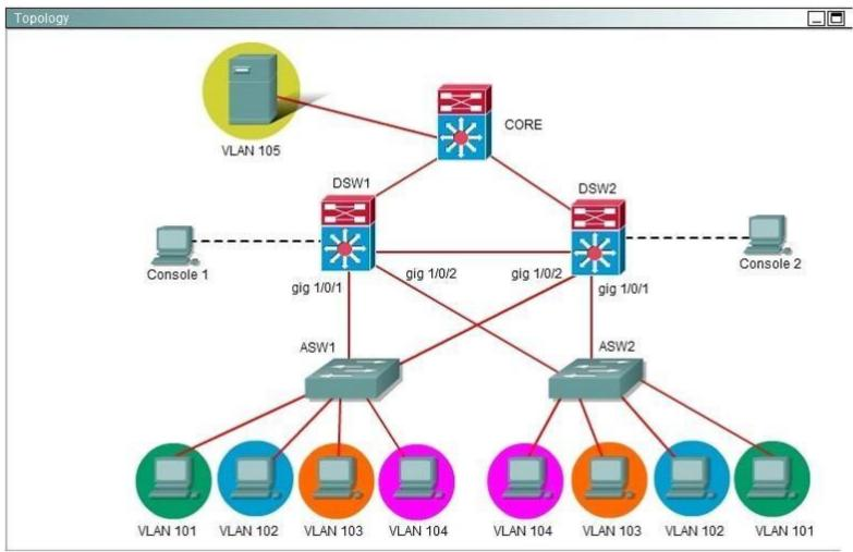
If GigabitEthemet1/0/1 on DSW2 is shutdown, what will be the resulting priority value of the VLAN 105 HSRP group on router DSW2?
