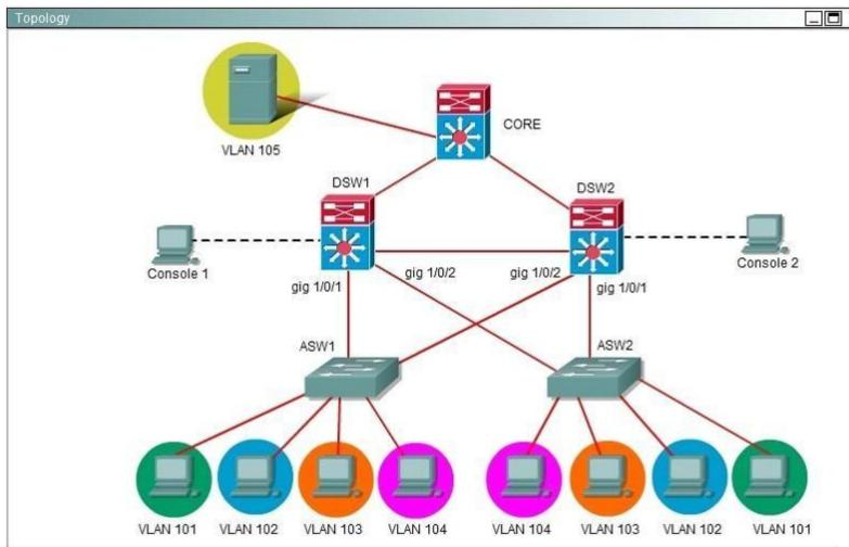
During routine maintenance, it became necessary to shut down the GigabitEthernet1/0/1 interface on DSW1. All other interfaces were up. During this time, DSW1 remained the active device for the VLAN 102 HSRP group. You have determined that there is an issue with the decrement value in the track command for the VLAN 102 HSRP group. What needs to be done to make the group function properly?
