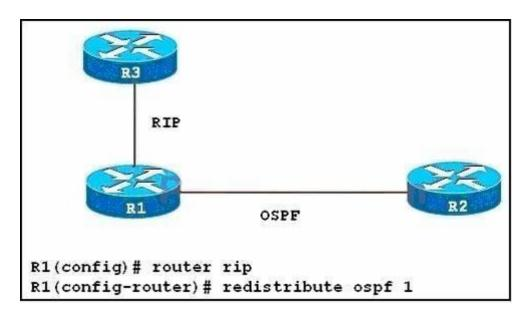
Routers R1 and R2 have been configured to operate with OSPF. Routers R1 and R3 have been configured to operate with RIP. After configuring the redistribution between OSPF and RIP on R1, no OSPF routes are distributed into RIP. What should be done to correct this problem?
