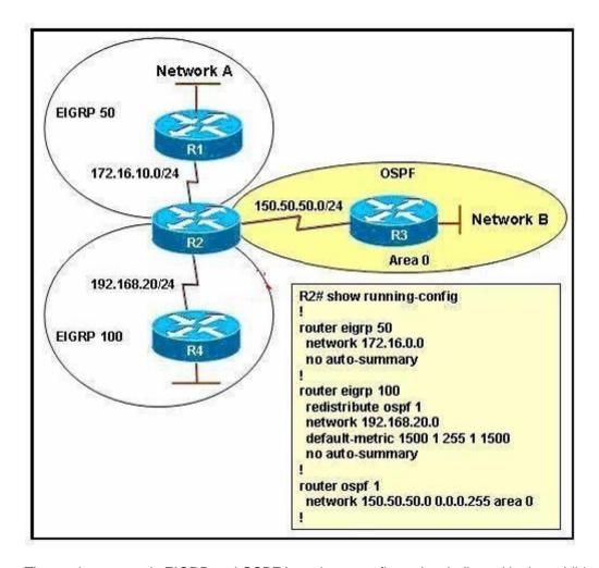
The routing protocols EIGRP and OSPF have been configured as indicated in the exhibit. Given the partial configuration of router R2, which network will be present in the routing table of R4?
