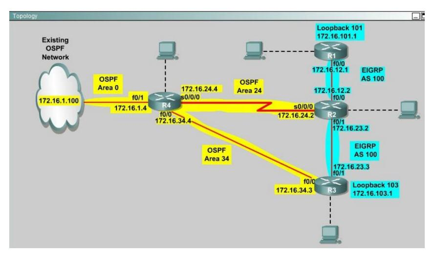
Correct Answer: Answer: First we need to find out 5 parameters (Bandwidth, Delay, Reliability, Load, MTU) of the s0/0/0 interface (the interface of R2 connected to
