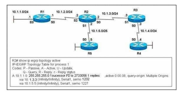
EIGRP had converged in AS 1 when the link between router R1 and R2 went down. The console on router R2 generated the following messages:
