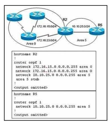
On the basis of the configuration provided, how are the Hello packets sent by R2 handled by R5 in OSPF area 5?
