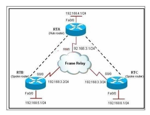
Router RTA is the hub router for routers RTB and RTC. The Frame Relay network is configured with EIGRP, and the entire network is in autonomous system 1. However, router RTB and RTC are not receiving each other's routes. What is the solution?
