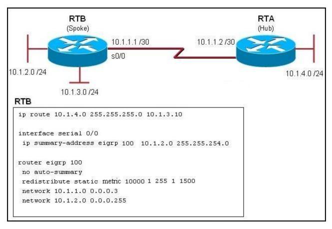
Which router configuration command can be given that will restrict router RTB from sharing its routing information with router RTA?
