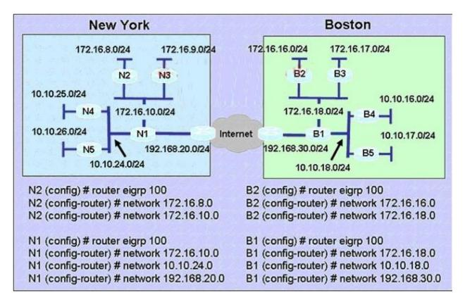
A Boston company bought the assets of a New York company and is trying to route traffic between the two data networks using EIGRP. The show command output shows that traffic will not flow between the networks. As a network consultant, you were asked to modify the configuration and certify the interoperability of the two networks. For traffic to flow from subnet 172.16.8.0/24 to the 172.16.16.0/24 subnet.
