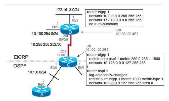
EIGRP has been configured on router D. Router C is performing mutual redistribution between EIGRP and OSPF. While verifying that the redistribution is functioning properly, you discover that while router C has all of the EIGRP routes in its routing table, router A does not have any routes from the EIGRP domain. What on router C may be the cause of the problem?
