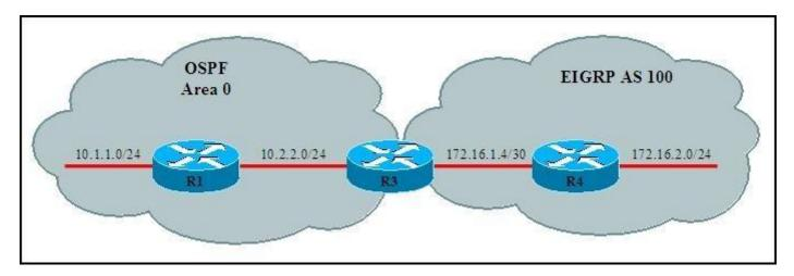
Refer to the topology diagram R3 is redistributing the EIGRP routers into OSPF. What will the EIGRP routes appear in the routing table of R1?
