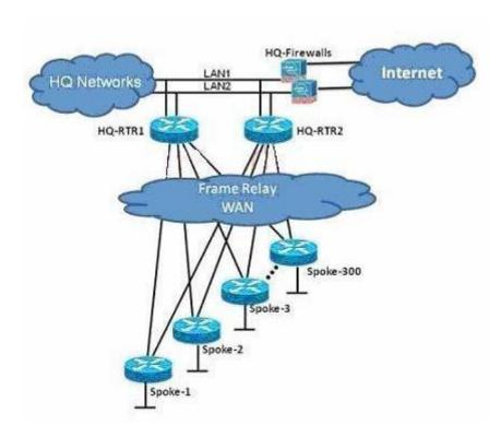
The Route.com company is running EIGRP between all the routers. Currently, if one of the LAN links (LAN1 or LAN2) at the headquarters flaps (goes up and down), the HQ-RTR1 and HQ-RTR2 routers will experience high CPU usage and have a long EIGRP convergence time. As the new network administrator, you are asked to investigate this situation and determine if there is a quick way to resolve this issue.
