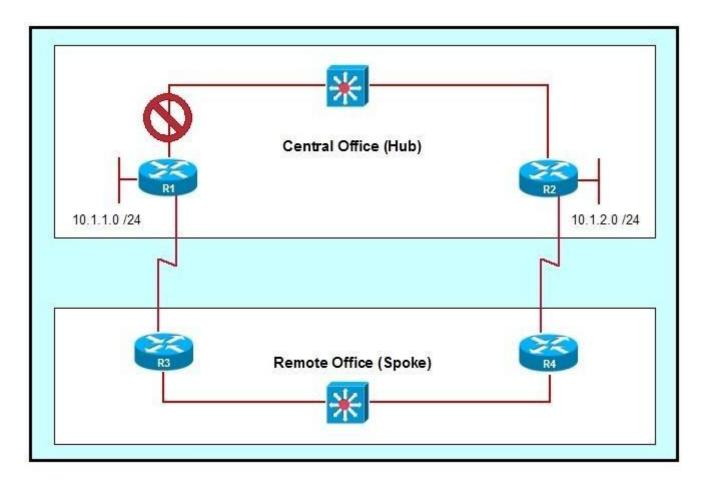
Network administrators have set up a hub and spoke topology with redundant connections using EIGRP. However, they are concerned that a network outage between Router R1 and Router R2 will cause traffic from the 10.1.1.x network to the 10.1.2.x network to traverse the remote office links and overwhelm them. What command should be used to configure the spoke routers as EIGRP stub routers that will not advertise connected networks, static routes, or summary addresses?
