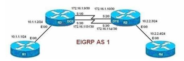
When you examine the routing tables of R1 and R4, you are not able to see the R1 Ethernet subnet on the R4 routing table. You are also not able to see the R4 Ethernet subnet on the R1 routing table.
