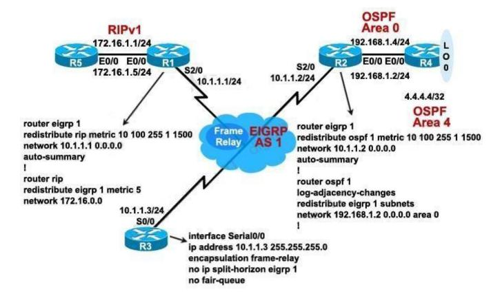
Looking at the topology diagram and the partial router configurations shown, which statement is true?
