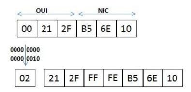
Once the above is done, we have a fully functional EUI-64 format address. Reference: https://supportforums.cisco.com/document/100566/understanding-ipv6-eui-64-bit-address
