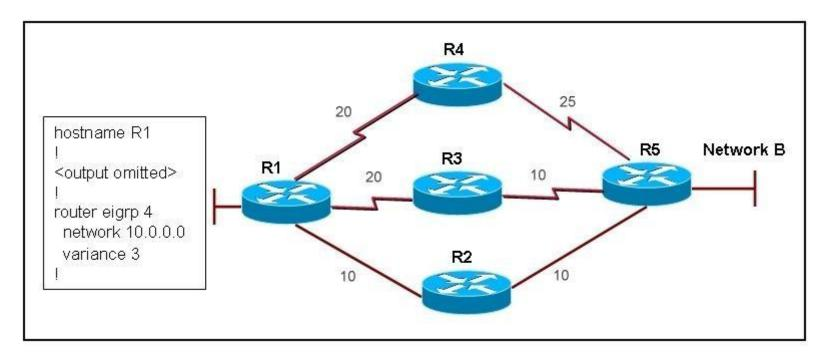
On all routers in the network, EIGRP has been configured for load balancing across the three links. However, traffic destined for Network B from R1 is only load balanced over paths R1- R2-R5 and R1-R3-R5. What is the cause of the problem?
