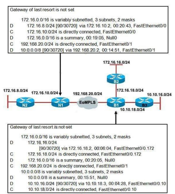
A Boston company bought the assets of a New York company and is trying to route traffic between the two data networks using EIGRP over EoMPLS. As a network consultant, you were asked to verify the interoperability of the two networks.
