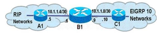
Which three commands should be used on router B1 to redistribute the EIGRP AS 10 routes into RIP? (Choose three.)
