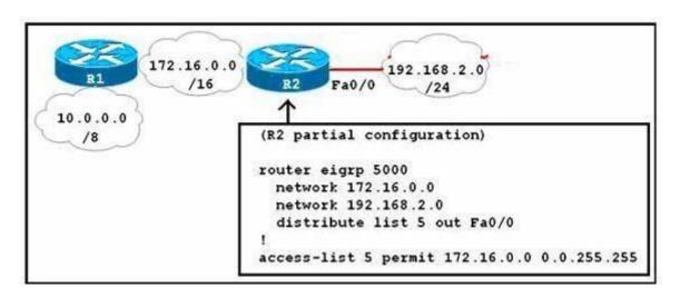
R1 and R2 have been configured to share routing information via EIGRP. What will be the result of the configuration section shown for R2?
