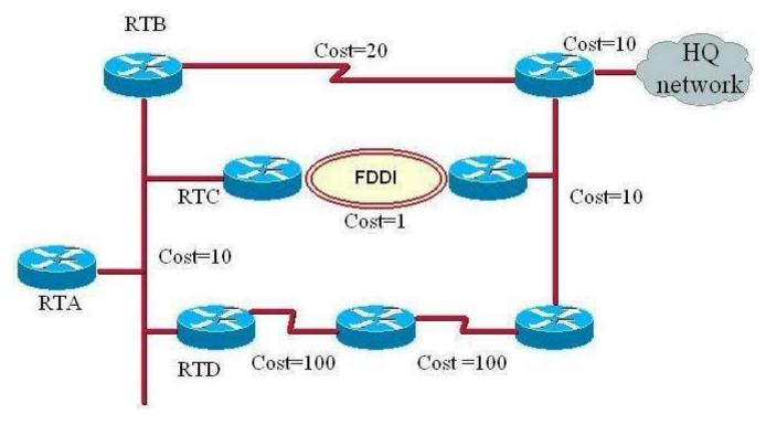
Routers in the Diagram are configured with EIGRP. If RTB and RTC fail, which action will RTA take with respect to the HQ network?
