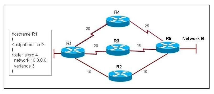
On all routers in the network, EIGRP has been configured for load balancing across the three links. However, traffic destined for Network B from R1 is only load balanced over paths R1- R2-R5 and R1-R3-R5. What is the cause of the problem?
