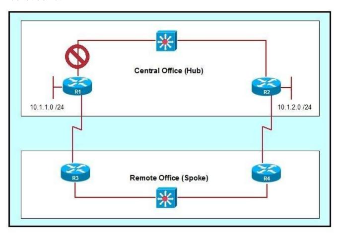
Network administrators have set up a hub and spoke topology with redundant connections using EIGRP. However, they are concerned that a network outage between Router R1 and Router R2 will cause traffic from the 10.1.1.x network to the 10.1.2.x network to traverse the remote office links and overwhelm them. What command should be used to configure the spoke routers as EIGRP stub routers that will not advertise connected networks, static routes, or summary addresses?
