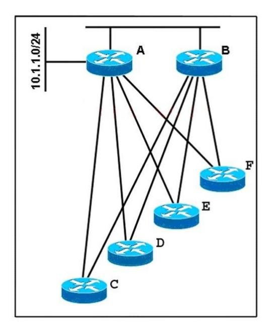
In a redundant hub-and-spoke deployment using EIGRP, what feature can be used to ensure that routers C through F are not used as transit routers for
