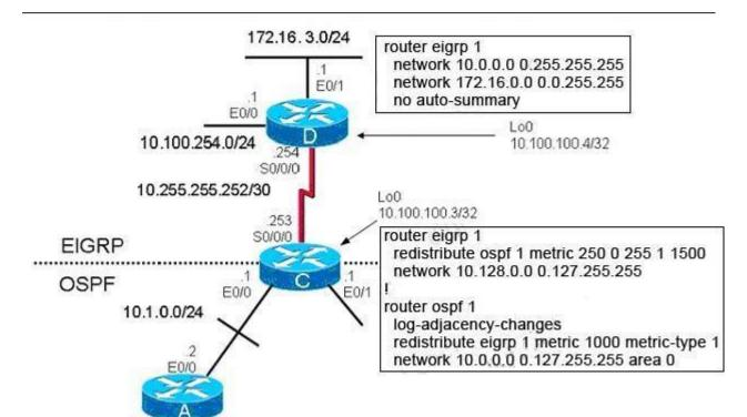
EIGRP has been configured on router D. Router C is performing mutual redistribution between EIGRP and OSPF. While verifying that the redistribution is functioning properly, you discover that while router C has all of the EIGRP routes in its routing table, router A does not have any routes from the EIGRP domain. What on router C may be the cause of the problem?
