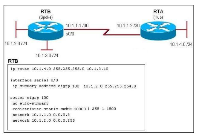
Which router configuration command can be given that will restrict router RTB from sharing its routing information with router RTA?
