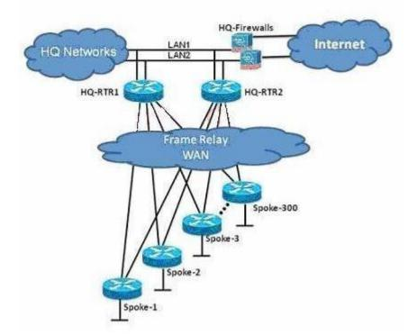
The Route.com company is running EIGRP between all the routers. Currently, if one of the LAN links (LAN1 or LAN2) at the headquarters flaps (goes up and down), the HQ-RTR1 and HQ-RTR2 routers will experience high CPU usage and have a long EIGRP convergence time. As the new network administrator, you are asked to investigate this situation and determine if there is a quick way to resolve this issue. Which is the most important thing that you can quickly verify first to resolve this issue?
