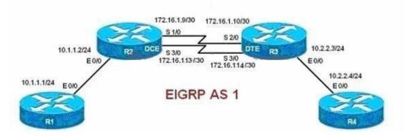
When you examine the routing tables of R1 and R4, you are not able to see the R1 Ethernet subnet on the R4 routing table. You are also not able to see the R4 Ethernet subnet on the R1 routing table.
