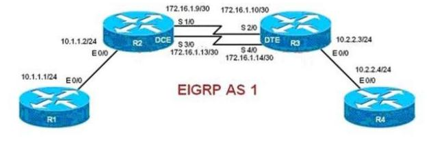
The actual speed of the serial links between R2 and R3 are 256 kb/s and 512 kb/s. When configuring EIGRP on routers R2 and R3, the network administrator configured the bandwidth of both serial interfaces to 512 kb/s.
