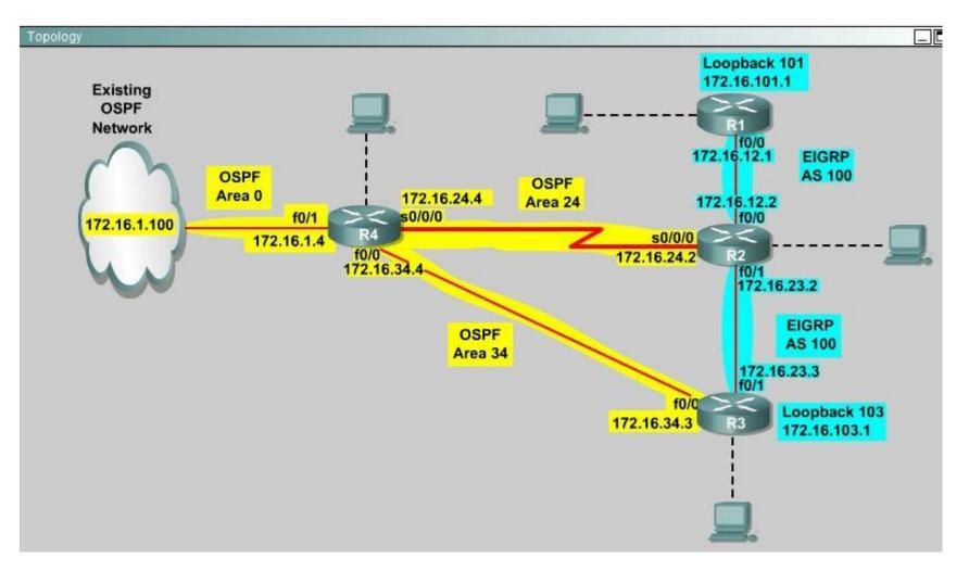
Correct Answer: Answer: First we need to find out 5 parameters (Bandwidth, Delay, Reliability, Load, MTU) of the s0/0/0 interface (the interface of R2 connected to R4) for redistribution: Section: Layer 3 Technologies Explanation
