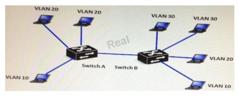
The network consists of two IP ProVision Switches with routing disabled. How should the network administrator configure the link between Switch A and Switch B to ensure all hosts can communicate to all the other hosts within their respective VLANs?
