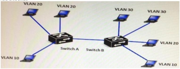
The network consists of two IP ProVision Switches with routing disabled. How should the network administrator configure the link between Switch A and Switch B to ensure all hosts can communicate to all the other hosts within their respective VLANs?
