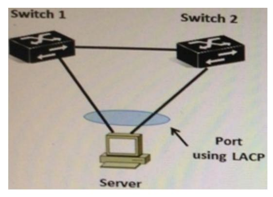
The server shown in the exhibit is configured for dynamic LACP. There is only one link between Switch 1 and Switch 2. Which HP switching solution should the network administrator implement?
