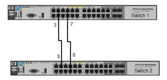
VLAN1: Ports 1,3,5,8-24 (untagged) VLAN 10: Ports 2,4,6,7 (tagged)
