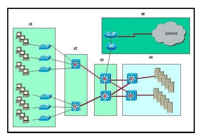
Refer to the exhibit. A standard Layer 2 campus network design is pictured. Which numbered box represents the core layer?
