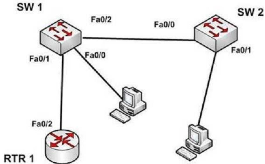
With the exception of frames traveling on the native VLAN, data frames crossing a trunk link must be frame tagged over the link to identify the VLAN that sourced the frame. The receiving switch sees the VLAN ID, and uses this information to forward the frame appropriately. 802.1q and ISL are the two possible frame tagging methods between Cisco switches. In summary, some facts about access and trunk ports:
