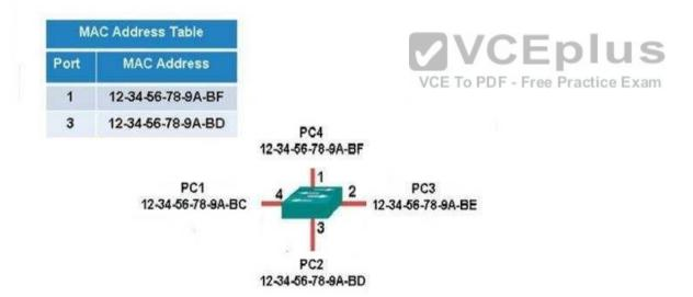
Which of the following frames will be flooded to all ports after it is received by the switch?
