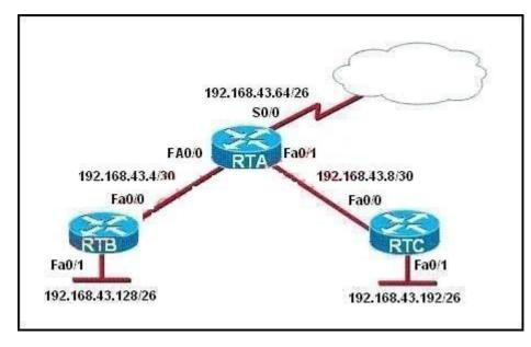
For security reasons, information about RTA, including platform and IP addresses, should not be accessible from the Internet. This information should, however, be accessible to devices on the internal networks of RTA.
