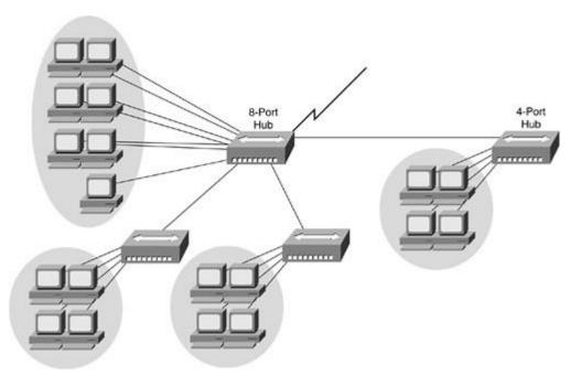
If the hubs in the graphic were replaced by switches, what would be virtually eliminated?
