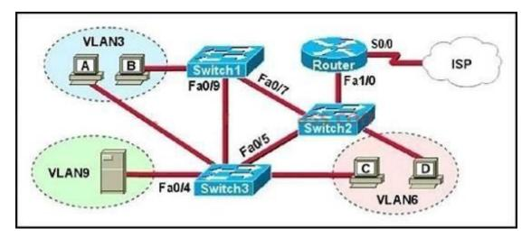
A problem with network connectivity has been observed. It is suspected that the cable connected to switch port Fa0/9 on Switch1 is disconnected. What would be an effect of this cable being disconnected?
