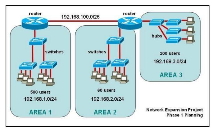
The junior network support staff provided the diagram as a recommended configuration for the first phase of a four-phase network expansion project. The entire network expansion will have over 1000 users on 14 network segments and has been allocated this IP address space. 192.168.1.1 through 192.168.5.255 192.168.100.1 through 192.168.100.255
