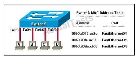
The exhibit is showing the topology and the MAC address table. Host A sends a data frame to host D. What will the switch do when it receives the frame from host A?
