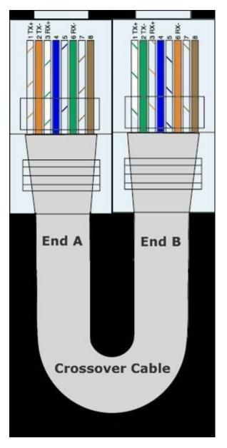
The wire scheme that is shown is terminated at each end with an RJ-45 connector. What cable type does the wire diagram represent?
