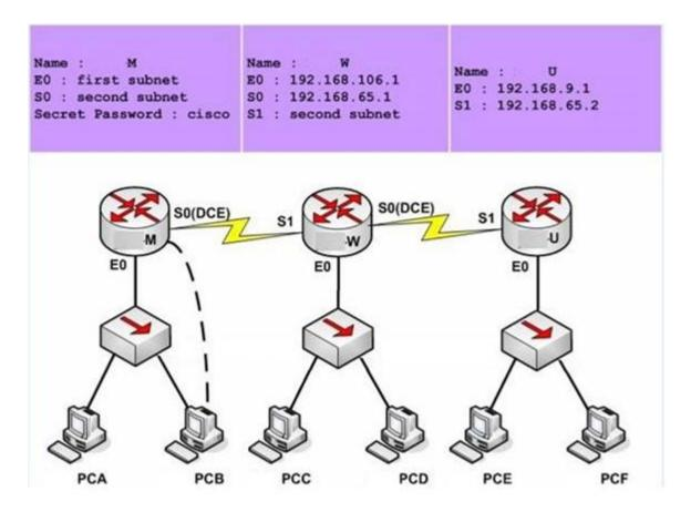
NotE. The OSPF process must be configured to allow interfaces in specific subnets to participate in the routing process.
