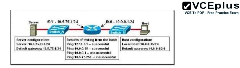
A technician is troubleshooting a host connectivity problem. The host is unable to ping a server connected to Switch\_A. Based on the results of the testing, what could be the problem?
