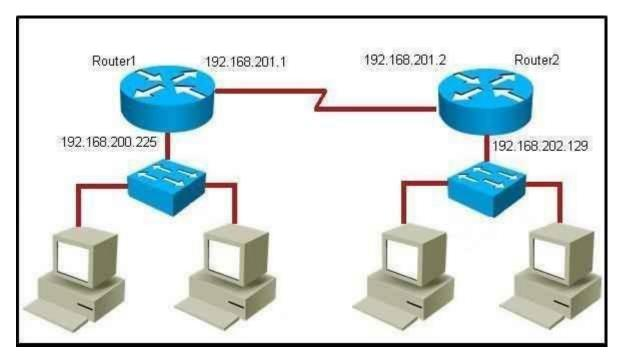
Which command would you use to configure a static route on Router1 to network 192.168.202.0/24 with a nondefault administrative distance?
