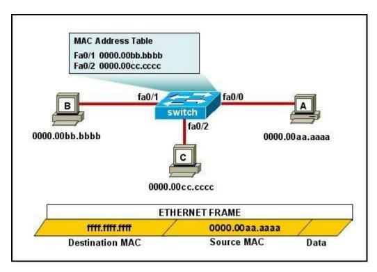
The MAC address table is shown in its entirety. The Ethernet frame that is shown arrives at the switch. What two operations will the switch perform when it receives this frame? (Choose two.)
