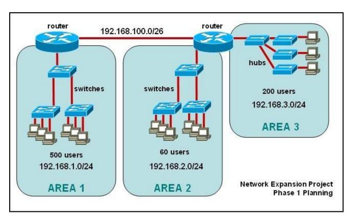
The junior network support staff provided the diagram as a recommended configuration for the first phase of a four-phase network expansion project. The entire network expansion will have over 1000 users on 14 network segments and has been allocated this IP address space. 192.168.1.1 through 192.168.5.255 192.168.100.1 through 192.168.100.255
